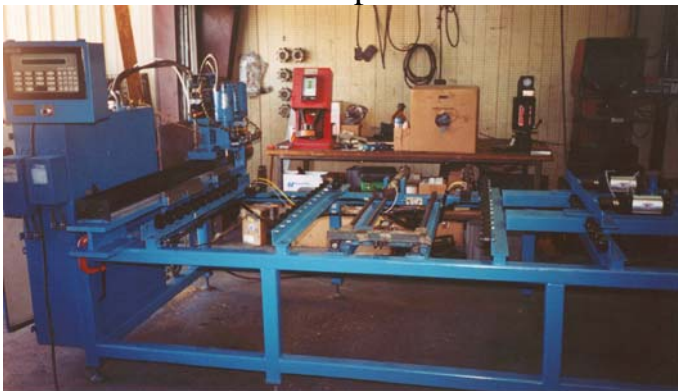
Elevator door drill & tap machine
