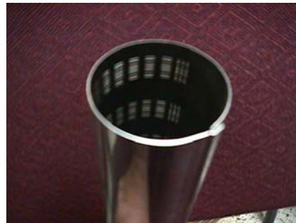
Roll form a tube and form an air tight seam from a flat blank
